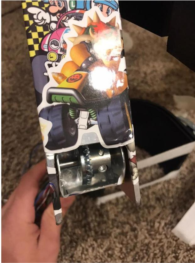
Figure 4: Gear connection inside the tube
